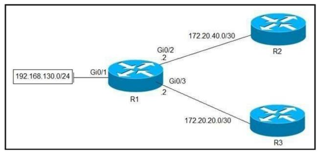
Which configuration configures a policy on R1 to forward any traffic that is sourced from the 192.168.130.0/24 network to R2?
