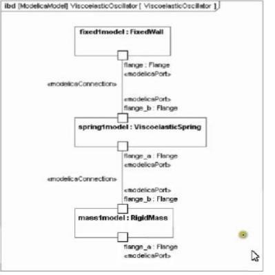
Assume that all stereotypes required by the SysML-Modehca Transformation specification (if any) have been applied but are not necessarily shown here Assume that FixedWall. ViscoelasticSpring. and RigidMass are fully defined in a Modelica library.
